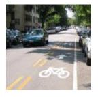
**Contra-flow bicycle lanes** allow bicyclists to ride in the opposite direction of motor vehicle traffic. They convert a one-way traffic street into a two-way street: one direction for motor vehicles and bikes, and the other for bikes only. Contra-flow
