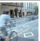
**Two-way cycle tracks** are physically separated cycle tracks that allow bicycle movement in both directions on one side of the road.
