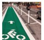
**One-Way Protected Cycle Tracks** are at street level and use a variety of methods for physical protection from passing traffic.
